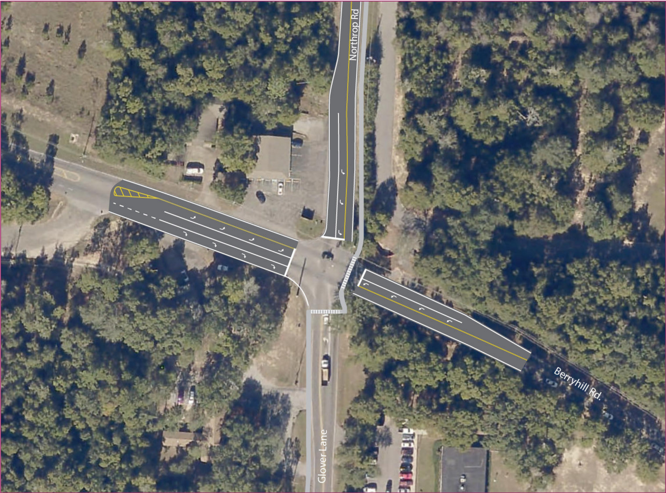
Figure 20. Proposed Pedestrian Crossing Treatment for the Glover Lane/Northrop Road at Berryhill Road Intersection
