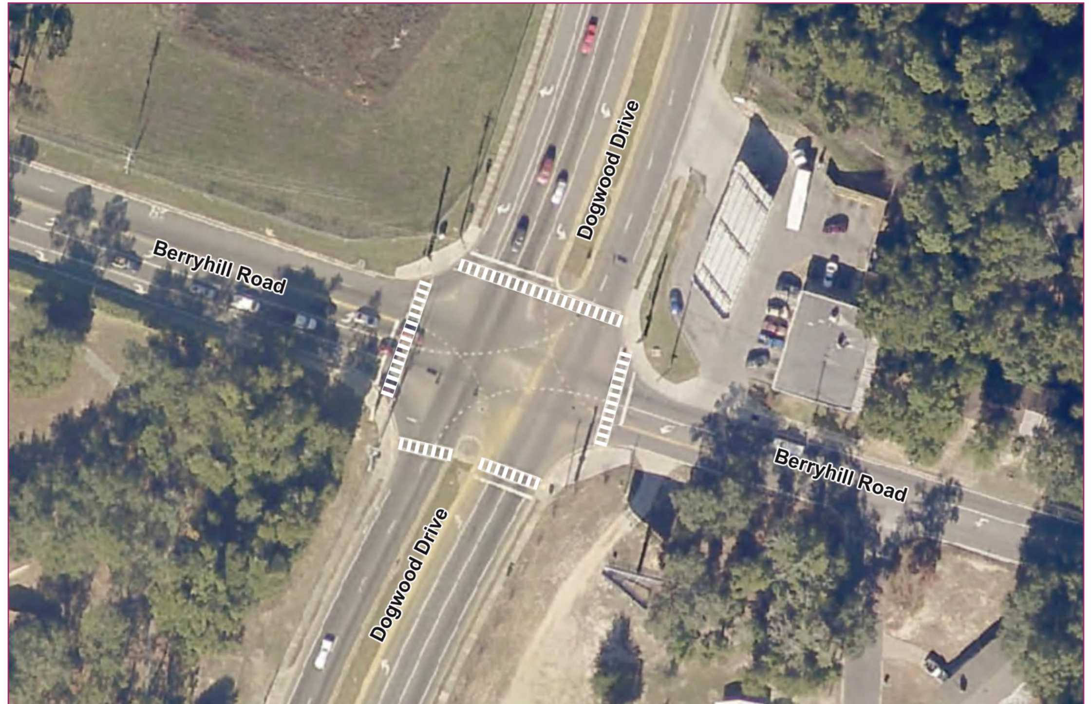
Figure 21. Conceptual Rendering of Proposed High-Emphasis Crosswalks at the Intersection of Berryhill Road and Dogwood Drive
