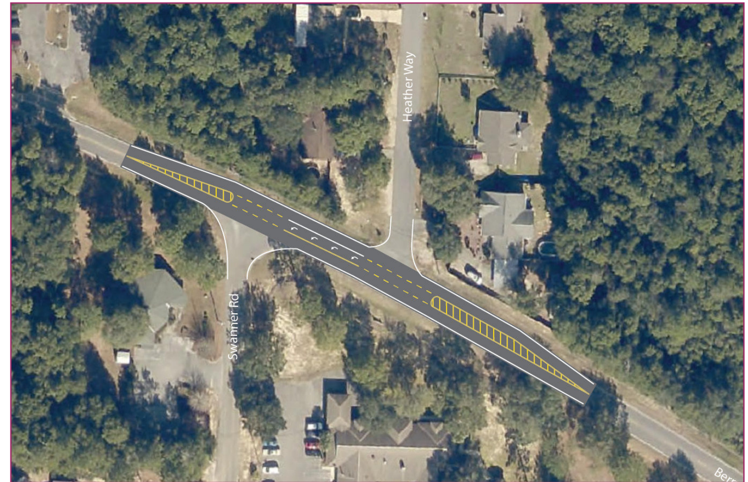
Figure 16. Conceptual Rendering of Proposed Turn Way at Swanner Road/Heather Lane
