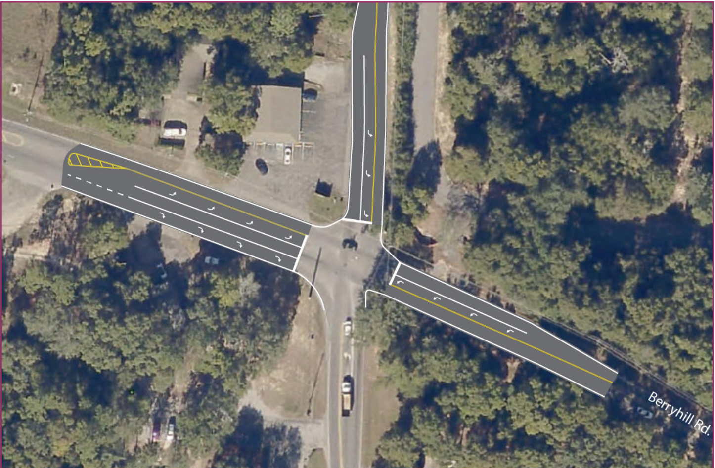
Figure 19. Conceptual Rendering of Proposed Turn Lane Extension
