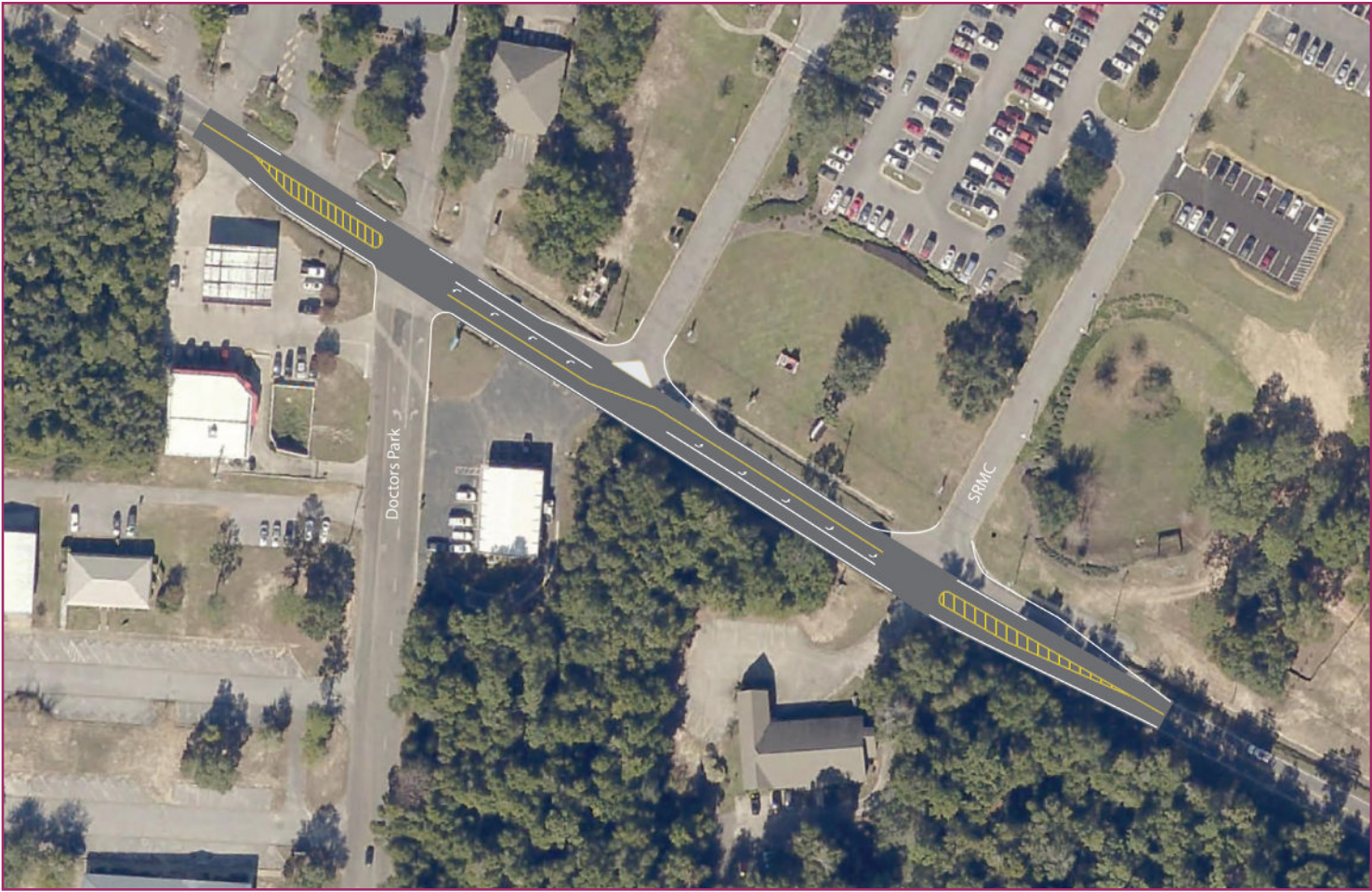
Figure 17. Conceptual Rendering of Proposed Turn Lane at SRMC
